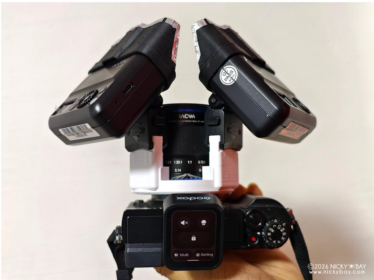
Top left: Front view of the setup, showing the UV-bandpass filter on each modified flash mounted on the custom 3D-printed flash holder. Top right: Side view. Bottom: Top view showing the custom flash mount. - Nicky Bay -
